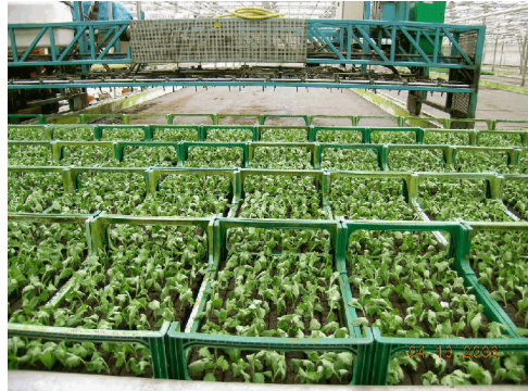
Transport robot shown, in rear, The robot can pickup and place the carrier trays, automatically treat the cuttings using the Spray Drip Down Method, and cover the trays with plastic..
